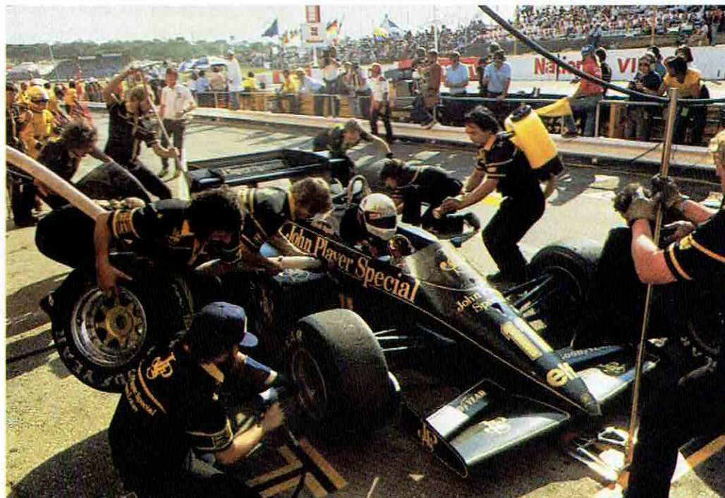
It's all systems go at Elio's race pit stop. The back pack collects any overflow from the water tank vent.
